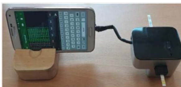
Fig. 1. Photo of manufactured prototype device of min-size portable urine analyzer.
